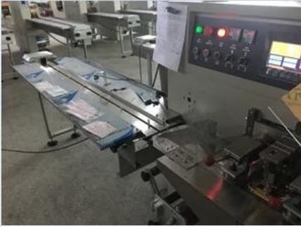
**1.Packed item go through the platform by manule or automatic.The Platform is make according different packed item**
