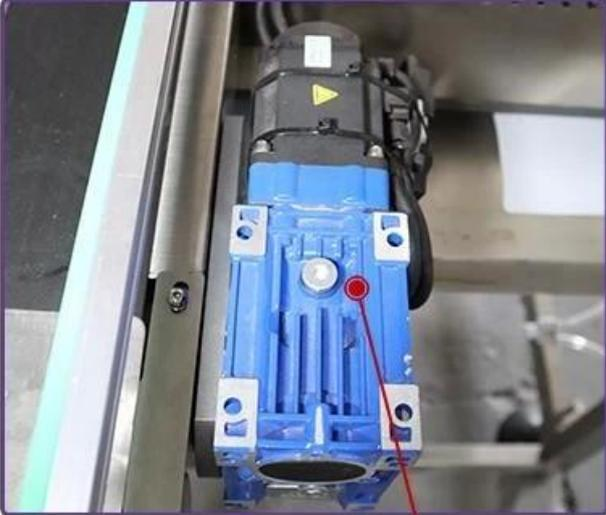
Conveyor belt servo motor
