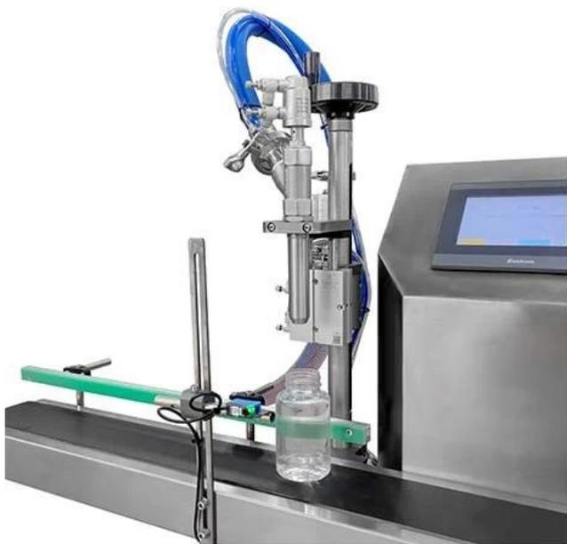
Cylinder (equipped with a leak stop valve)
