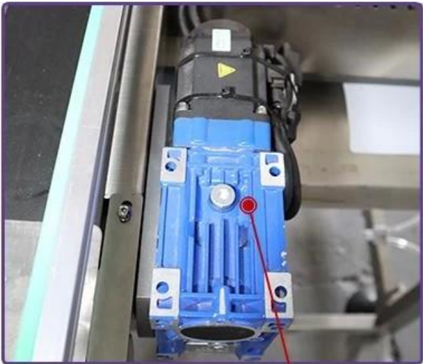
Conveyor belt servo motor
