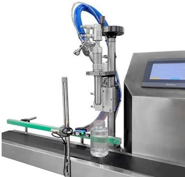
Cylinder (equipped with a leak stop valve)
