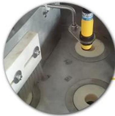
**Electric eye tracing & cup metering**
