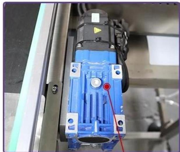
Conveyor belt servo motor
