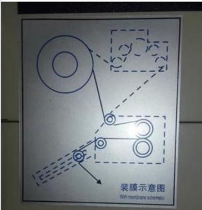
**3.Film schematic diagram to left the film placing more easy and clear**
