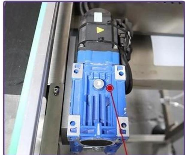
Conveyor belt servo motor
