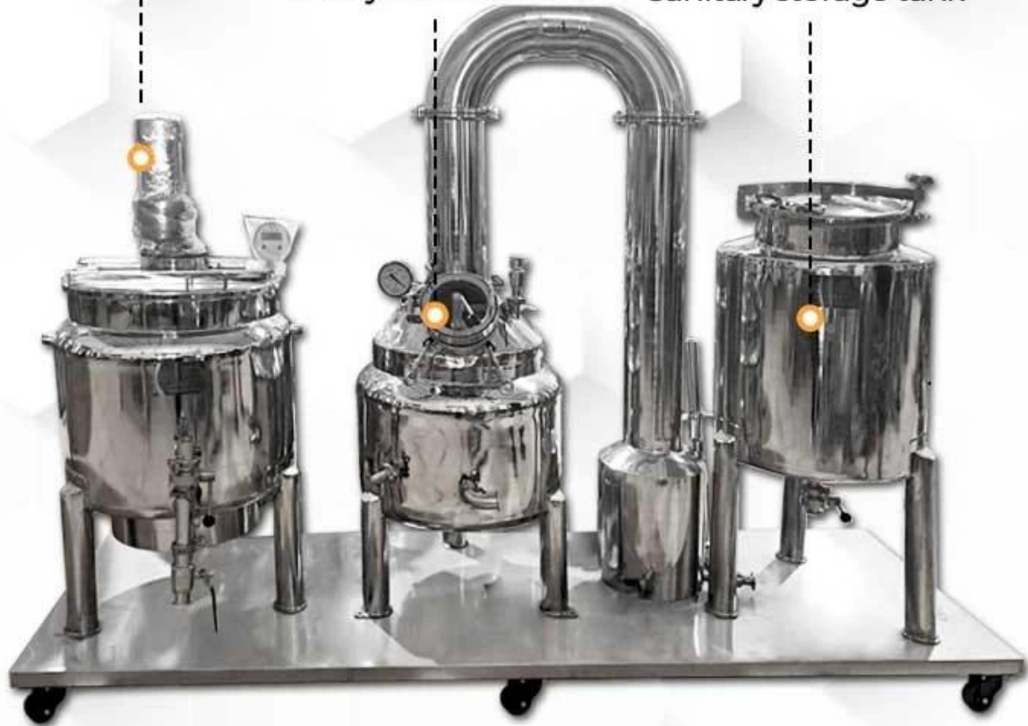
Preheating cylinder Honey concentrator Sanitary storage tank
