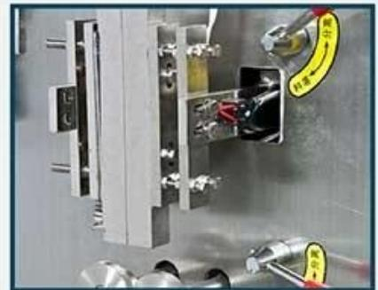
**Longitudinal sealing structure**
