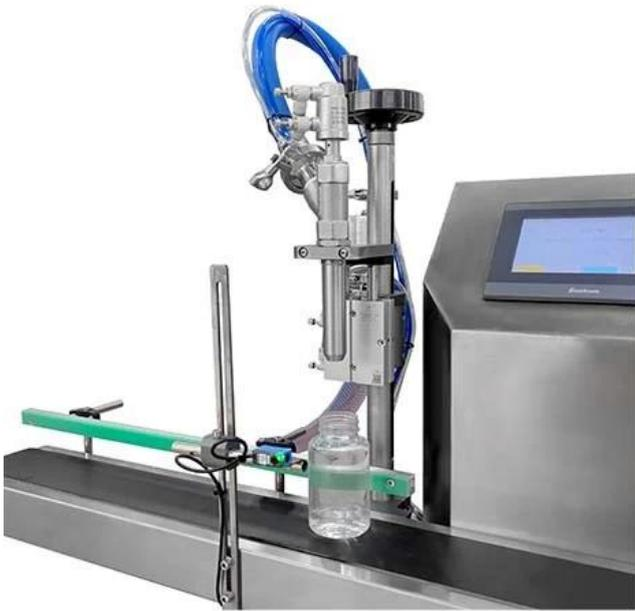
Cylinder (equipped with a leak stop valve)
