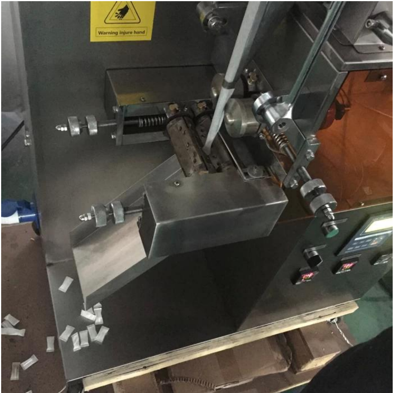
Cutting and sealing
