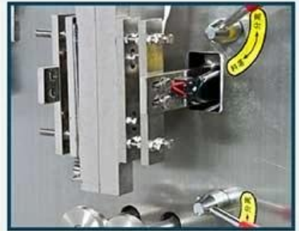
Longitudinal sealing structure
