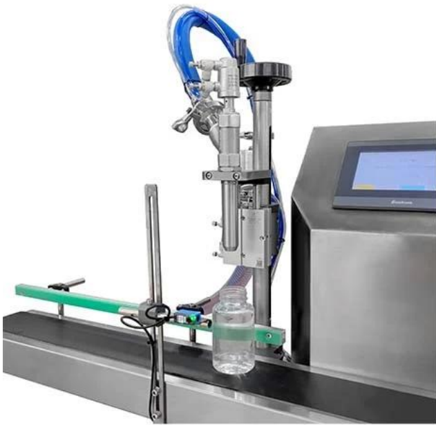
Cylinder (equipped with a leak stop valve)
