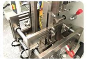
Four Side Sealing Mold
