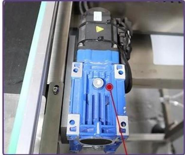
Conveyor belt servo motor
