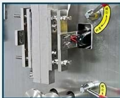
Longitudinal sealing structure
