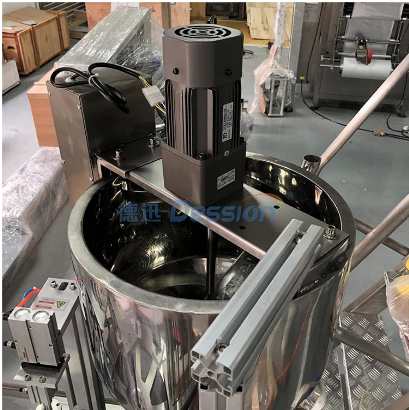
Hopper and heating stirring device
