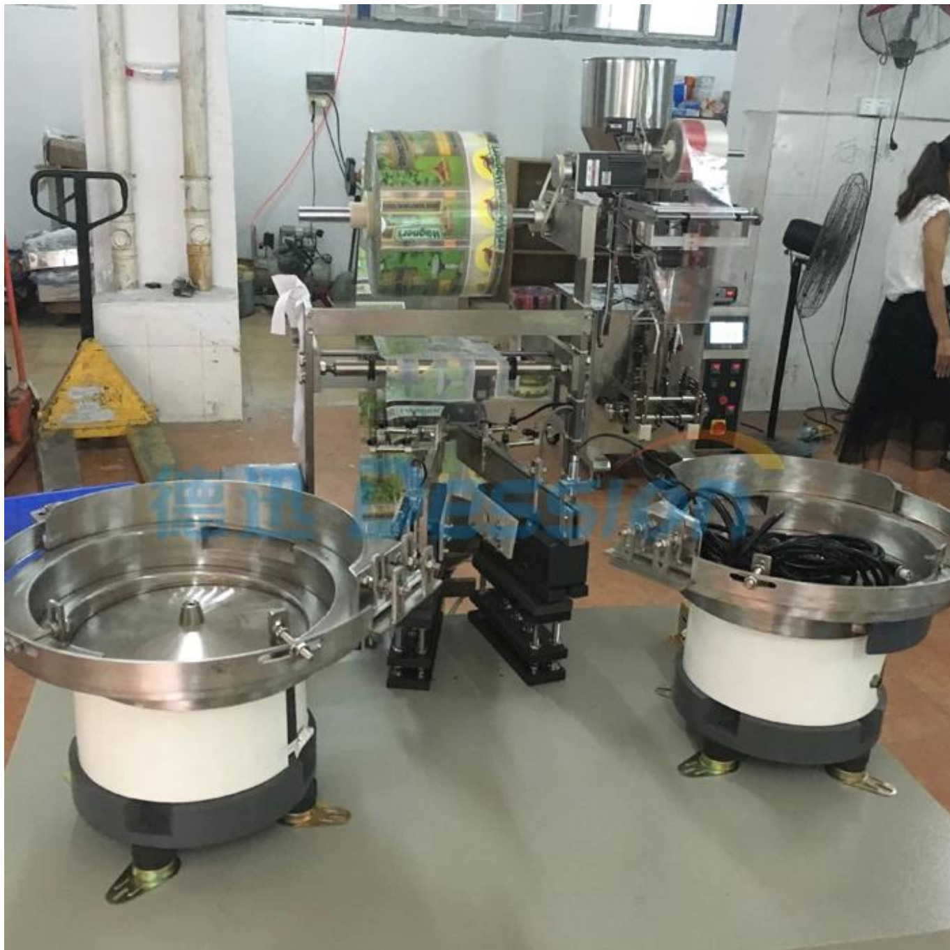
Vibration plate for Coffee Capsule Put in and turn around
