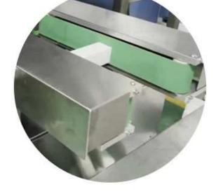
Automatically fold the ear to seal the box
