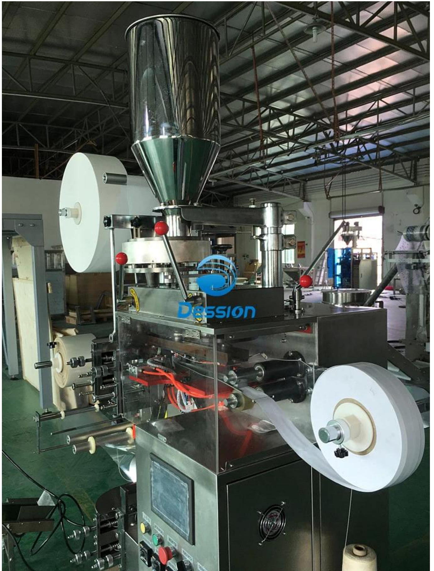
Machine Process for Tea Packer
