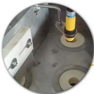
**Electric eye tracing & cup metering**
