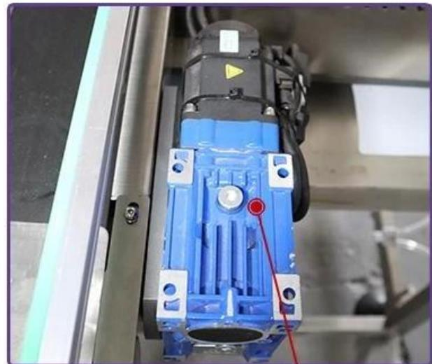
Conveyor belt servo motor
