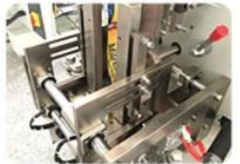
Four Side Sealing Mold
