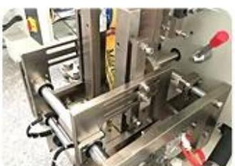
Four Side Sealing Mold
