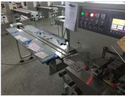
1.Packed item go through the platform by manule or automatic. The Platform is make according different packed item
