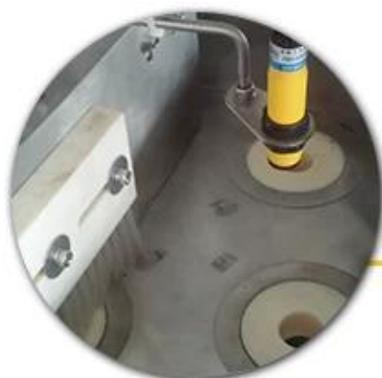
**Electric eye tracing & cup metering**
