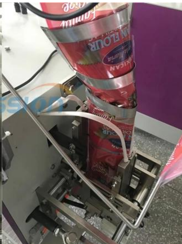
Figure 2. The process of the flour bag production
