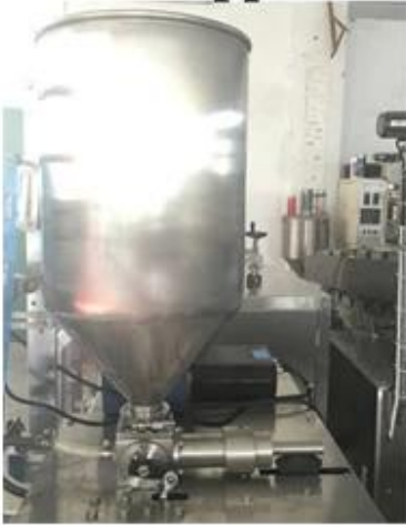
Sachet tomato ketchup package solution 20L hopper for liquid storage, can be customized
