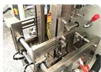
Four Side Sealing Mold
